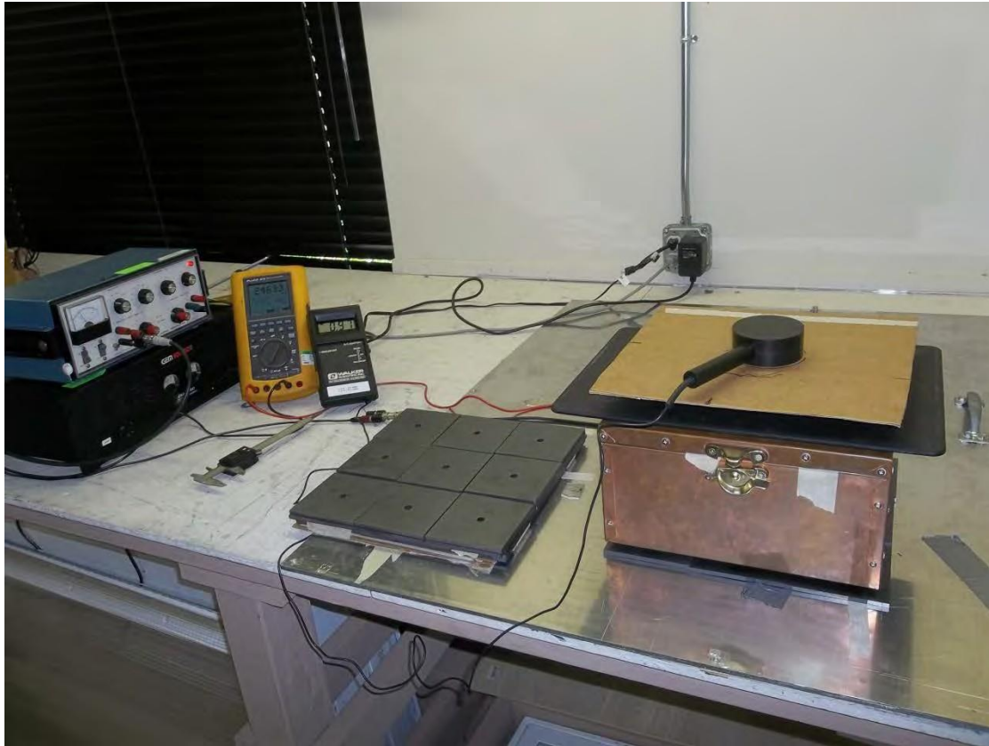
Figure 2. ELF EMR (Magnetic Component at 60 and 300 Hz) Test Configuration Photograph
